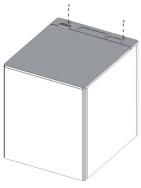
**2** Pull the indoor unit cover for upper piping outlet backward and remove it.
