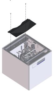
2 Remove the metal plugs (Heating coil connections) from the 3-way valve and the T-branch. If necessary, disconnect the 3-way valve motor (upper part) to ease the installation procedure.
