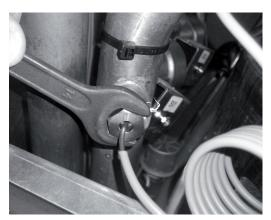
**5** Press two rings of the manometer rear side and remove it passing the capillary through the hole of the steel support.
