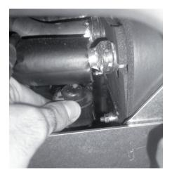
6 Replace the expansion valve coil by new ones by performing the procedures above in reverse way.
