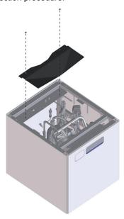
2 Remove the plastic plugs (space heating connections) from the 3-way valve and the T-branch. If necessary, disconnect the 3-way valve motor (upper part) to ease the installation procedure.
