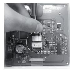
3 Replace LCD controller by a new one.
