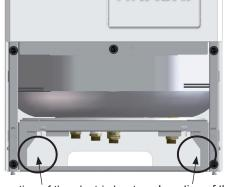
Location of the electric heater and thermistor cables LCD cable
