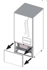
When reassembling, take into account that this cover is not symmetric. Upper and lower hooks are not at the same distance from the upper and lower cover edges.
