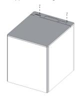
2 Pull the indoor unit cover for upper piping outlet backward and remove it.
