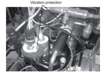
4 Remove the pressure sensors:
